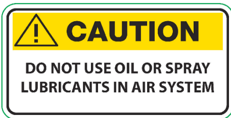
SPM301 ONLY! Do Not Use Oil In Air System
